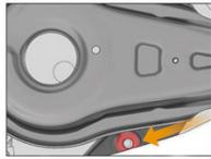
Install the rear ride height torque tool in the subframe hole.
